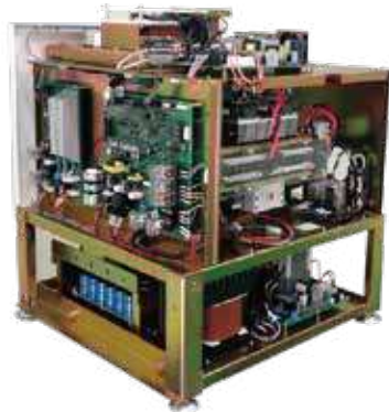
32kW / 40kW Super Capacitor Bank (PSU Generator)
